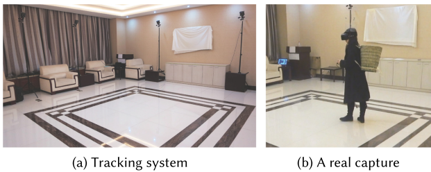
Fig. 10. Experimental setup. Eight motion capture cameras are used to track the users’ positions (a). During walking, the laptop and power supply are in the basket carried by users (b).
